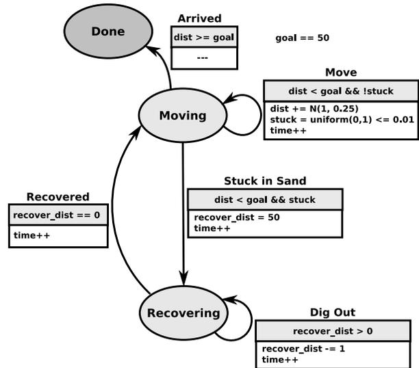
Figure 5: The stochastic simulation model for *Move*. This is used to simulate execution, and provides the state that is used for duration prediction during execution. In addition, this model is used offline to generate the observations used by the KDE-based predictor.
